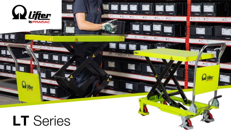
The scissor lift tables with foot-operated hydraulic pump are the ideal tools for a variety of lifting and loading operations and for use as "work station" to provide improved ergonomic conditions together with improved productivity. Available with 150-800 kg nominal capacity, single and double scissor for elevation up to 1300 mm, they represent the best solution for the manual load handling, combining functioning, cost saving, safety and health of operator during work.
